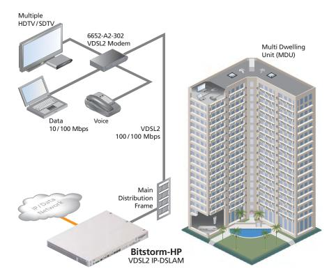
Bitstorm-HP is ideally suited for deployment in Multi Dwelling Units and delivery of bandwidth intensive services such as HDTV, Video Conferencing, Interactive Gaming and symmetric business E-Line services. Bitstorm-HP supports dual Gigabit Ethernet uplinks which can be aggregated using standards based line aggregation protocol (LACP 802.3ad). This allows deep-fiber deployment and interface with Metro switches.
